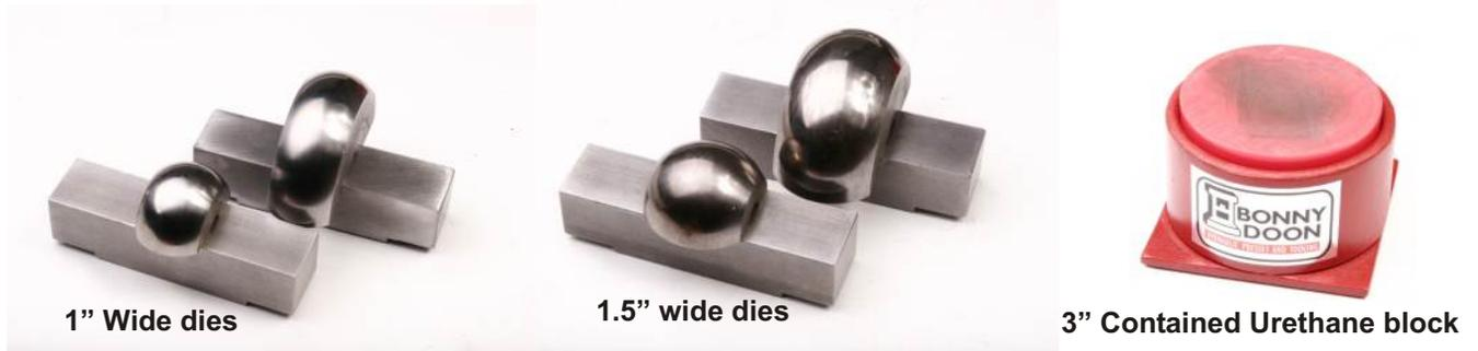
Note that there are two forming heads for each width--both formers in each pair have the same width and the radius is identical in each pair of formers. However, in each pair, one former has a long axial curve that is appropriate to the curve of the top of a wrist; the other former has a tighter axial curve that fits around the side of a wrist.
