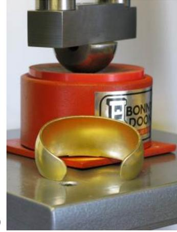
Move the metal strip about half an inch, and press again(2). Repeat until the entire strip has formed smoothly. It is helpful to watch the pressure gauge, and use the same pressure each time. It is better to press with light pressure using many strokes than to press with high pressure and few strokes.
