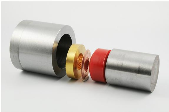
**Step 4 assembly - container, die, pre-formed metal, 95 duro urethane, pusher**
