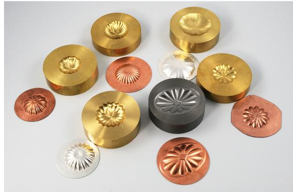
**Examples of brass and steel dies and pressed metal**
